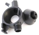
Powder is leaking or the AutoThrow is jamming and the tension screw will not fix it. Remove the tension screw and clean the inside surfaces of stray powder. Apply graphite dry lubricant if possible. Reassemble and readjust the tension screw.
